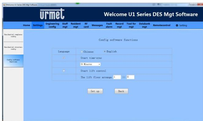
Activate system timing to set the timing interval.
